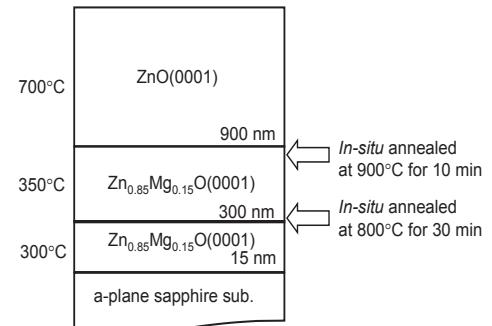
Fig.1 Schematic diagram of a sample structure. スタイル名 : Fig\_01 8pt
